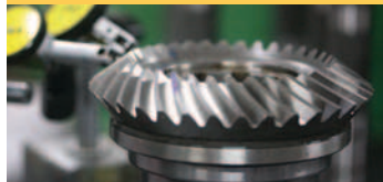
Hypoid Gears with 4-tooth pinions
