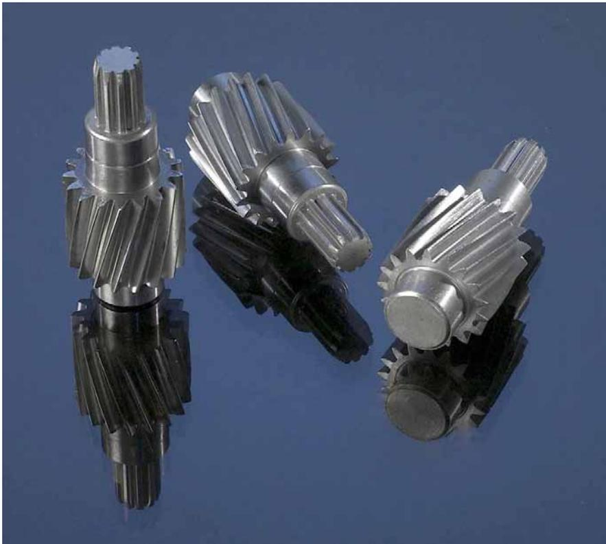
(lead) of 15 microns and a profile error of less than 30 microns. Additionally, this gear has an accurately machined inside diameter (24 microns total tolerance) and locating face, enabling precise assembly.
