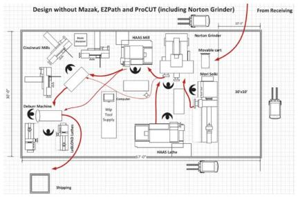
Figure 2 Material Flows in the Proposed Layout for the MP Cell (MPC).
