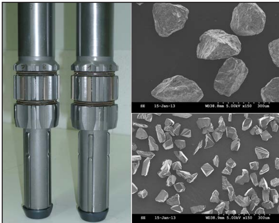
Figure 4 Hone tools with lower guides and CBN abrasive crystals (B213/B46).
