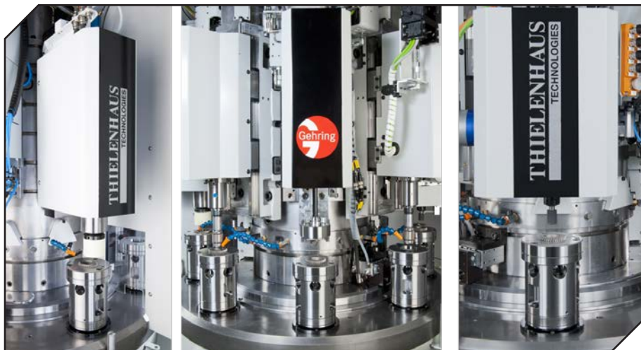
Figure 8 Machining stations for machining planetary gears.
