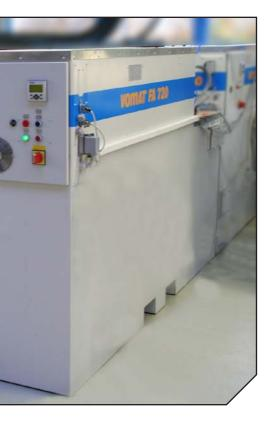
ing the backflush cycle the operator always has full oil flow. This allows for energy efficient, time optimized operation in sync with the customer's grinding machine. The Vomat FA 120 through 420 series machines with dimensions of  $1 \times 1 \times 1.6$  meters are also significantly smaller than comparable filtration systems on the market. This keeps transportation costs low, possibly reduces
