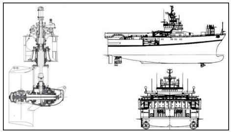
Figure 1 Positioning and design of the thruster (Ref. 16).
