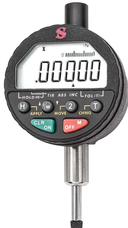
Numeric/ Analog AD model showing the two displays simultaneously.
