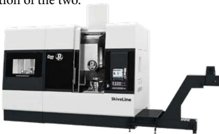
The SkiveLine has also been optimized for fully automatic series production: The work chambers of up to two gear centers are automatically supplied with tools via the automation cell, thus minimizing space and investment requirements compared with robot loading. Pittler Skiving also means that Pittler supplies the tools and clamps from a single source.
