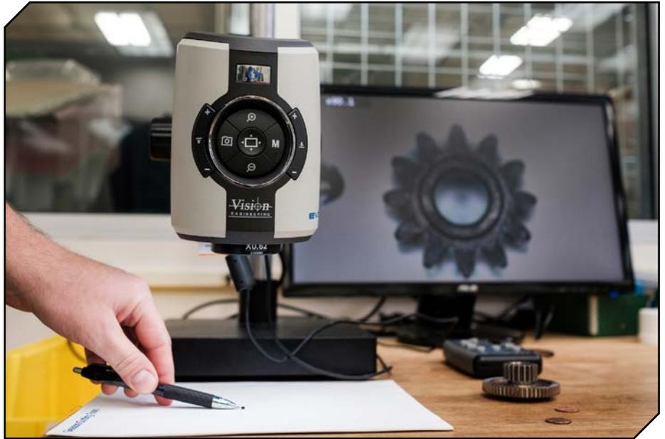
workpiece, or the smallest detail, at the touch of a button. It also has a 360° rotating viewer capability to reveal an angled all-round view of the part.
