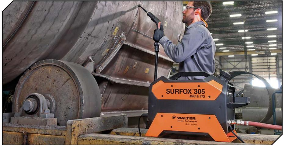
the surface, but this layer is compromised from the heat caused by welding,” says Jonathan Douville, senior product manager - Surfox, Finishing & Tooling. “Surfox 305 can safely, quickly, and effectively remove the heat tints caused by welding to help restore the corrosion resistance of stainless steel.”
