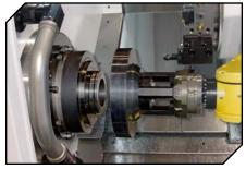
Positrol's Automation Chuck Change System can be installed on lathes, mills, balancers and gear equipment. It accommodates any drawbar and most common machine spindle sizes. Repeatability accuracy for the X, Y, and Z axes are within .0001" TIR and an angular repeatability within ±3 arc seconds. Sealed to account for chips and other contamination, Positrol's Automation Chuck Change offers low maintenance, faster changeovers and fully automated machining capabilities.
