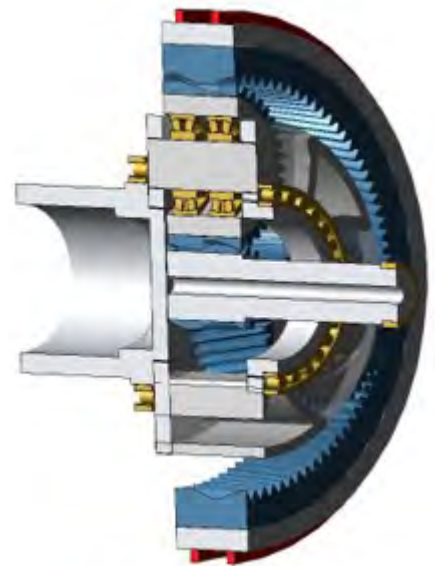
Figure 1 Example of a planetary stage (Source: FVA-Workbench 3D model).
