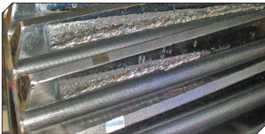
Figure 3 One-sided pitting on a sun pinion shaft in a wind turbine gearbox (Source: GearConsult).
