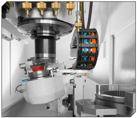
As compared to the typical cutter resharpening process, the new on-board unit is remarkably fast and simple. The machine's axes position the cutter to a grinding wheel. The integrated cutter sharpening unit then executes the necessary grinding strokes while the cutter performs the infeed and the indexing from tooth to tooth, all performed automatically and based on the new cutter geometry that exists after a certain number of gears has been cut (Courtesy Gleason).
