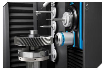
continuous, uninterrupted rotation of the component, the measurement time advantage increases with large numbers of teeth to up to 80 percent. It is not necessary to scan a large area of the gear with multiple revolutions.
