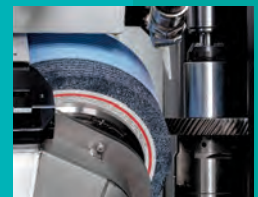
Toyo – Gear Generating Grinding
