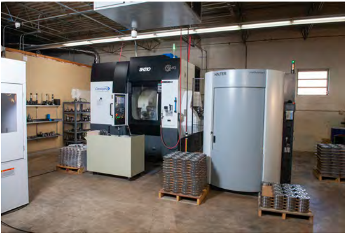
SMG's SH210 vertical hobbing machine, paired with Halter LoadAssistant automation, runs reliably unattended overnight, effectively adding second and third shifts.
