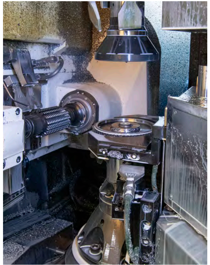
The SH210's 4-station ring loader automates loading and unloading, eliminating non-productive time and operator strain. Integrated chamfering/deburring during hobbing removes the need for manual downstream handling.
