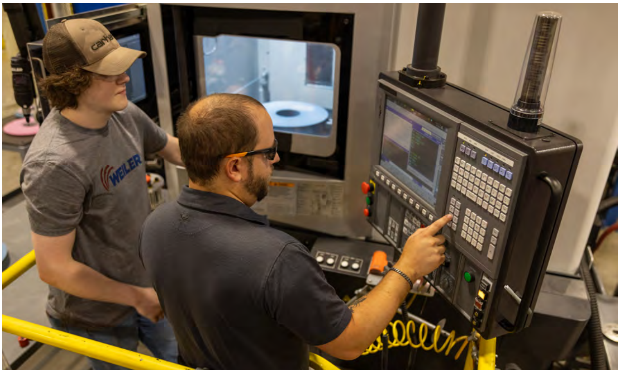
This image shows the cell where wheels are profiled as part of the Weiler Precision Express program, which cuts lead times for gear grinding wheels from months to weeks with on-demand wheel finishing.
