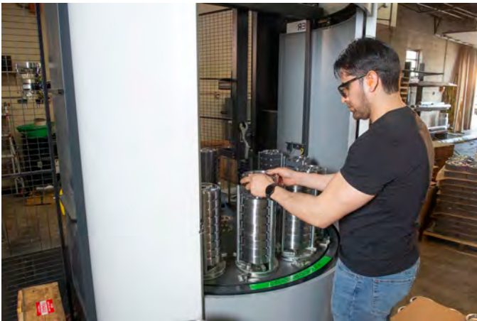
Operator loads the Halter's palletized stacker storage with gear blanks for completely automated, unattended hobbing overnight.
