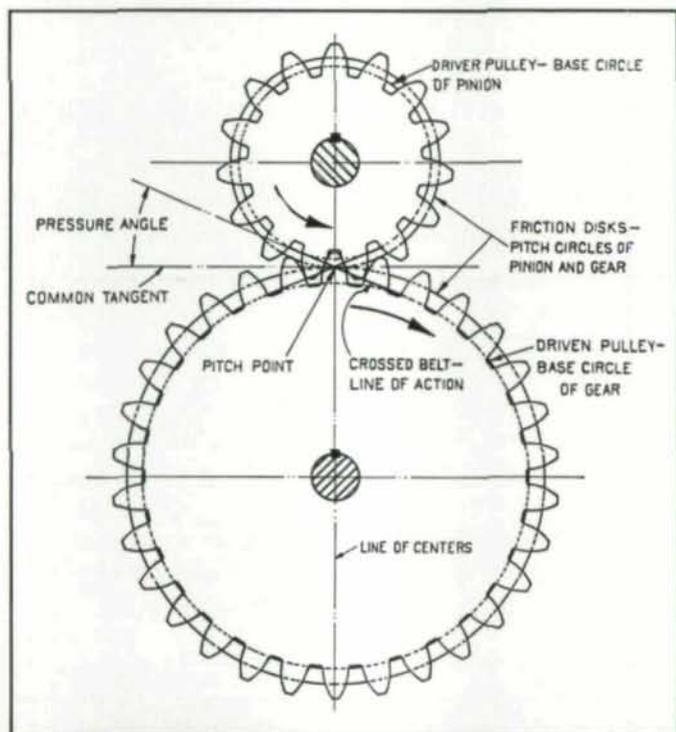
Fig. 4 — Diagram Showing Gears, Pulleys and Crossed Belt, Superimposed on Friction Disks, Illustrating Basic Gear Elements.
