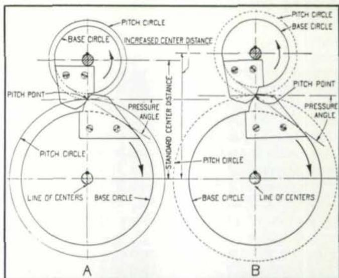
Fig. 5 — Diagram Illustrating That Changes in Center Distance Do Not Affect Velocity Ratio, or Conjugate Tooth Action.
