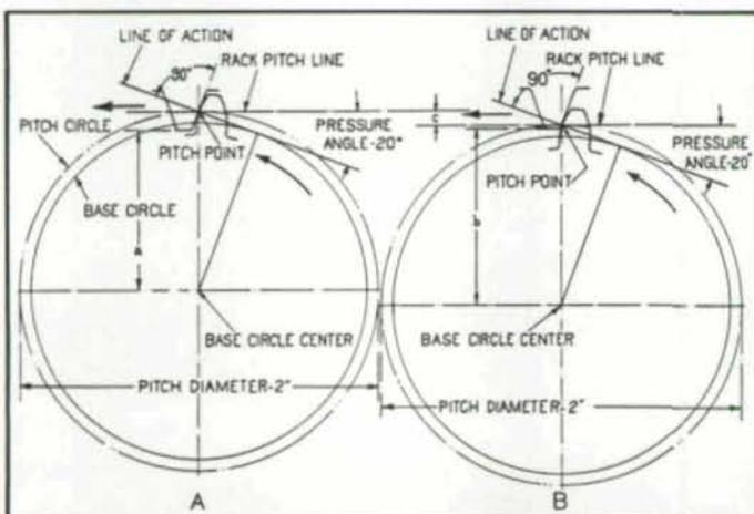
Fig. 10 — Diagram Illustrating That the Pressure Angle and Pitch Circle Diameter Do Not Change When a Gear Tooth Is Moved Closer to or Farther Away from a Rack.
