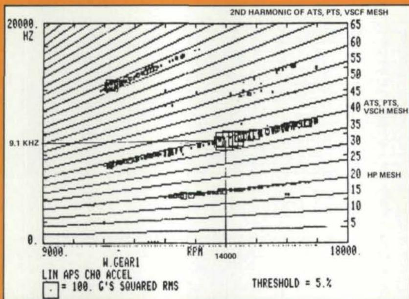
Fig. 5—(above) Excitation order diagram of baseline configuration
