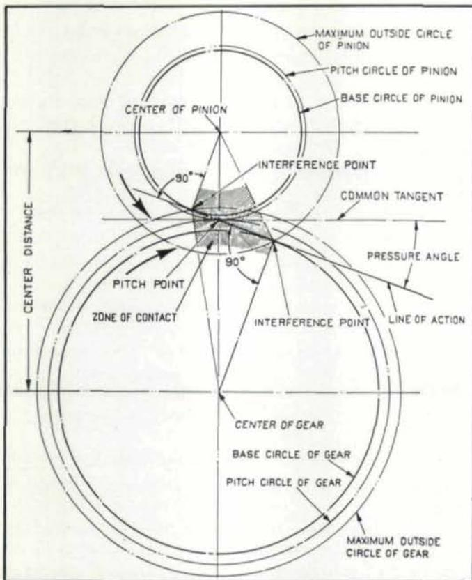
Fig. 11 — Diagram Presenting Principal Boundary Surfaces of Gear and Pinion, Showing Maximum Permissible Outside Diameters to Avoid Involute Interference.
