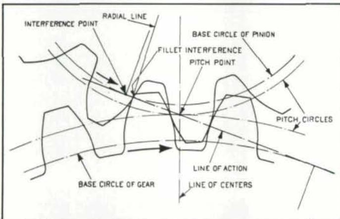
Fig. 16 — Diagram Illustrating Term Known as Fillet Interference. Gear Tooth Contacts Non-Involute Portion of Pinion Tooth Inside the Zone of Contact.
