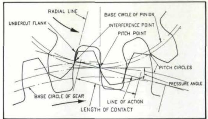
Fig. 13 — Diagram Showing Undercut Flank on Pinion Tooth to Avoid Involute Interference.
