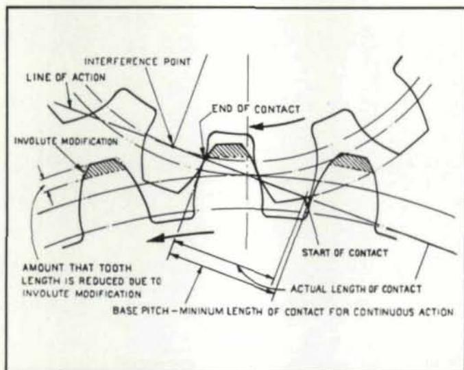
Fig. 19 — Diagram Illustrating Lack of Continuous Action Resulting from Involute Modification.
