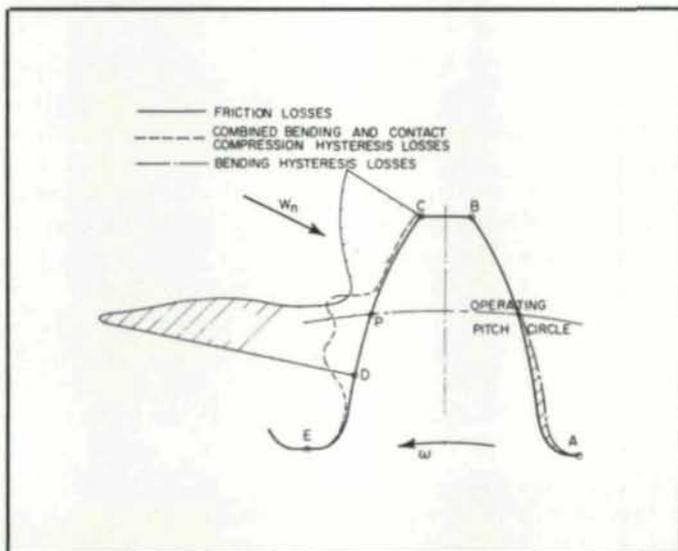
Fig. 1—Repartition of friction losses along gear profile.
