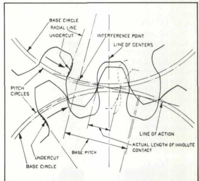
Fig. 18 — Diagram Illustrating Lack of Continuous Action Resulting from Undercutting of Flanks of Teeth. Also Due to Small Pressure Angle and Small Number of Teeth in Both Members.
