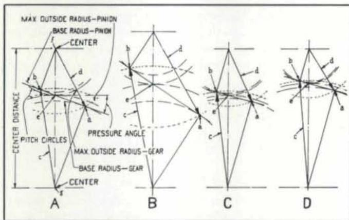
Fig. 7 — Diagram Illustrating That a Straight-sided Rack Tooth is the Proper Shape to Engage with an Involute Gear Tooth—Also That an Involute Contacting a Rack Transmits Uniform Linear Motion to the Rack.
