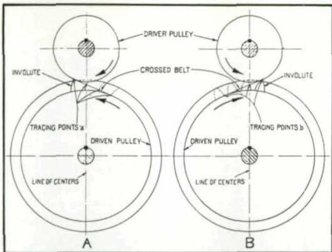
Fig. 3 — Diagram Showing How Equally-spaced Points on Crossed Belt Trace Successive Equally-spaced and Parallel Involute Profiles.
