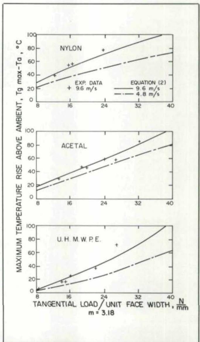
Fig. 7—Predicted Maximum temperature rise above ambient ( $T_{g_{max}} - T_a$ ) as a function of the tangential load per unit face width ( $W_t$ ) for two different speeds. Three materials, all: 8 pitch (3.175 module)
