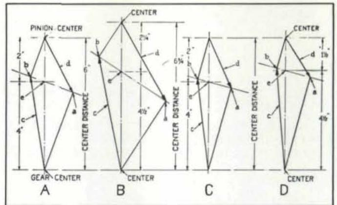
Fig. 8 — Diagram Illustrating Basic Elements of Involute Gearing.
