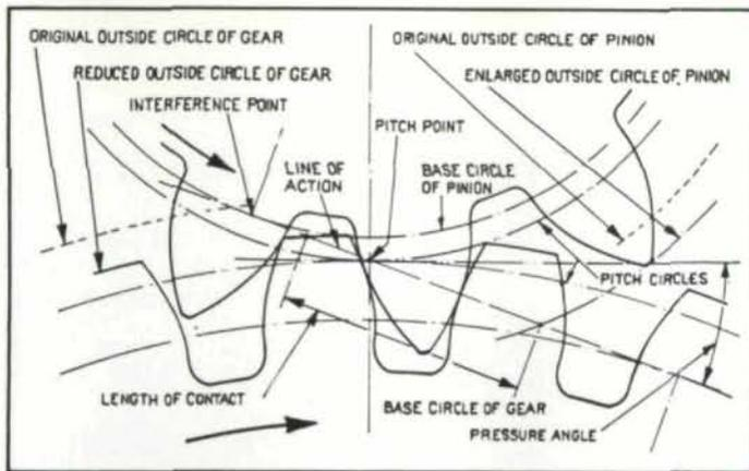
Fig. 15 — Diagram Illustrating Application of Long- and Short-Addendum, Coupled with Increased Pressure Angle to Avoid Involute Interference.
