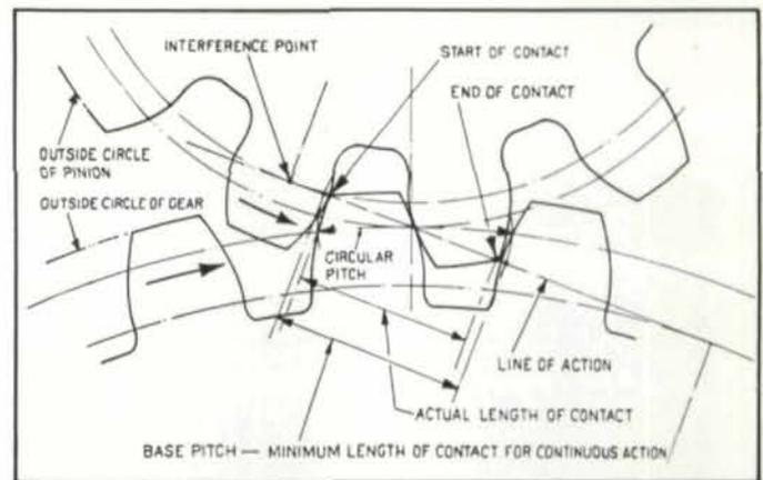
Fig. 17 — Diagram Illustrating Lack of Continuous Action as a Result of Shortened Teeth.
