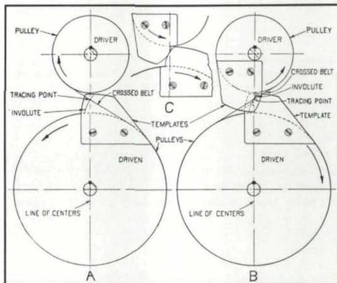
Fig. 2 — Diagram Illustrating That the Involute Is That Curve Traced by a Point on a Crossed Belt as It Moves from One Pulley to Another.
