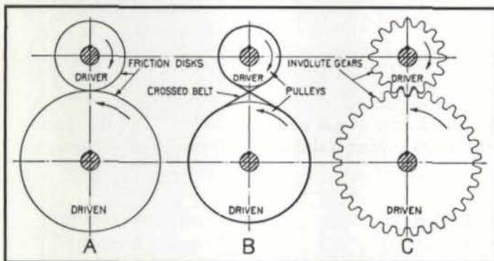
Fig. 1 — Diagram Illustrating Three Means for Transmitting Rotary Motion from One Shaft to Another.
