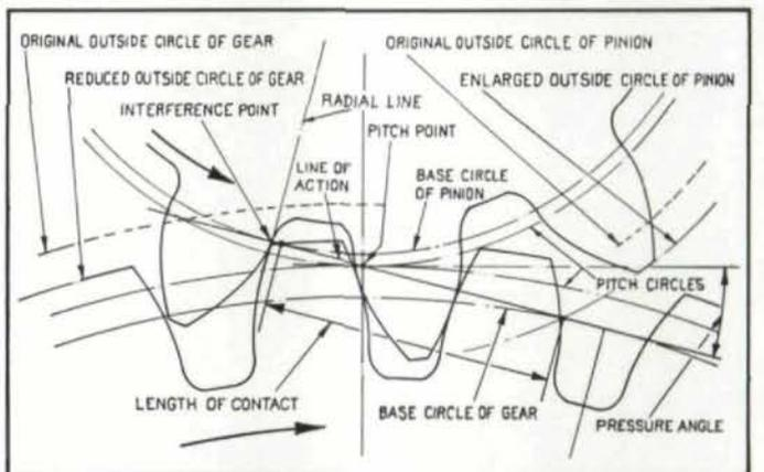
Fig. 14 — Diagram Illustrating Application of Long- and Short-Addendum Teeth to Avoid Involute Interference.
