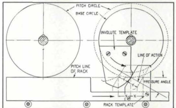
Fig. 9 — Similar Diagrams to Fig. 8, Except That Arcs Have Been Added to Indicate Pitch Circles, Base Circles, and Maximum Permissible Outside Radii of Gear and Pinion, Respectively.
