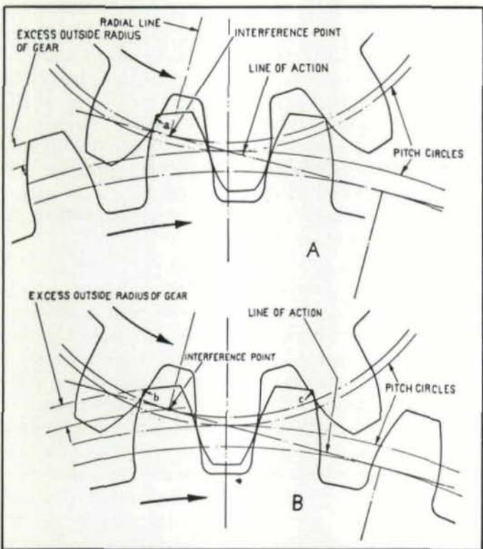
Fig. 12 — Diagram Illustrating Term Known as Involute Interference. Gear Tooth Contacts Non-Involute Portion of Pinion Tooth Outside the Zone of Contact.
