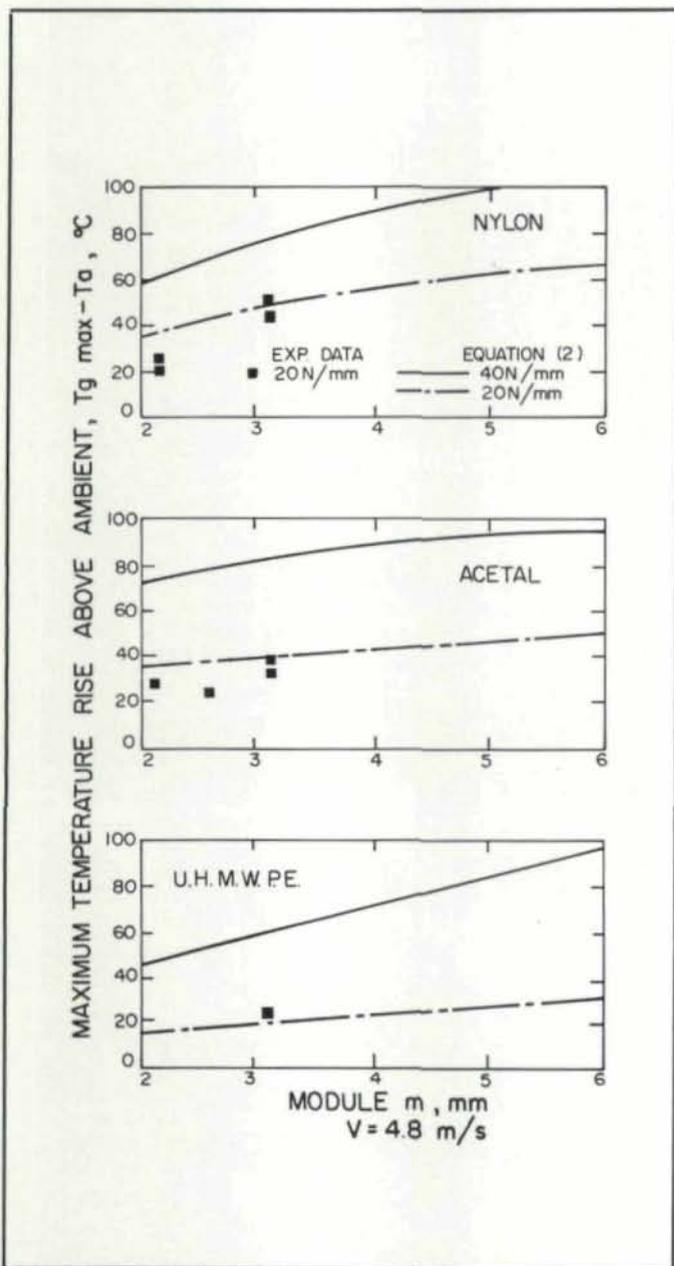
Fig. 8—Predicted Maximum temperature rise above ambient ( $T_{g\max} - T_a$ ) as a function of the module  $m$  for two different loads. Three materials, all 4.8 m/s pitch line velocity.
