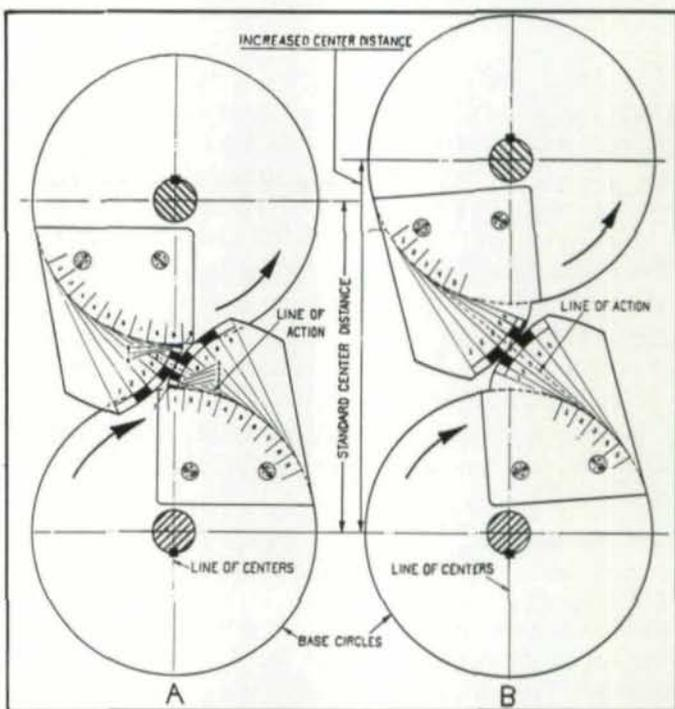
Fig. 6 — Diagram Illustrating Relative Slippage of Involute Gear Teeth.
