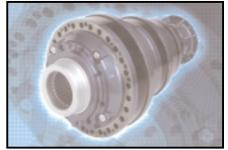
traction, marine and food processing industries. Available in eight sizes, the series contains four reduction stages and offers maximum nominal torque outputs up to 370,000 N-m.
