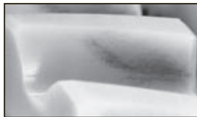
Figure 6—Tooth flank of nylon gear.
