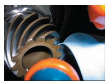
using a grinding wheel tip extension and a setover, to get a smooth blend of the ground to the unground root surface and clean up the root radius to the area of 30° tangent.
