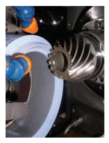
grinding profile surface just before its entrance into the grinding zone. Additional pipes are located behind the grinding zone and are directed opposite to the grinding speed to extinguish the sparks, which would burn into the wheel bond and get into the grinding zone.
