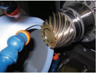
However, rejected parts and customer complaints are 1% or less for typical grinding production compared with 3-7% for lapping, depending on the requirements for certain jobs. Rejected gear sets include the cost of all previous operations plus the material. Consequently, the cost related to this difference in reject rate often makes grinding the more economical process.
