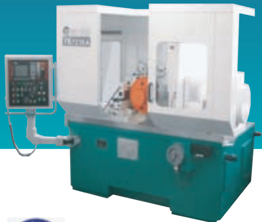
Worm Wheel Gear Grinder YK7236-A
