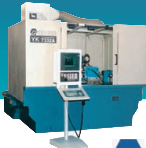
Form Wheel Gear Grinder YK7332-A
