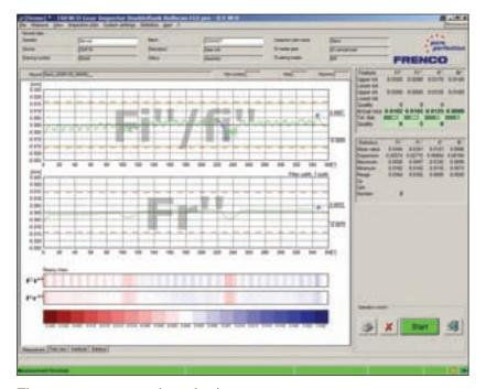
The measurement and evaluation software *Frenco Gear Inspector/FGI Pro* has been upgraded with new features. *FGI Pro* has an applicationoriented development and can be used for retrofitted Mahr and Hommel instruments.
