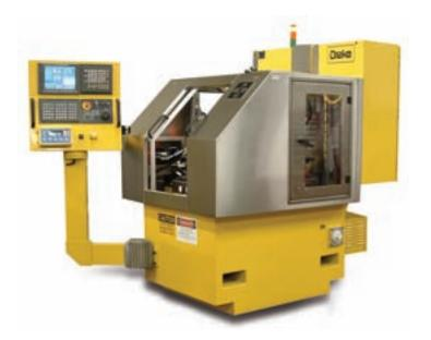
handles small batch production well. Steering Rack Milling Machines will also be on display. This auto-load production cell machine can mill racks in 35 seconds to a 0.4 Ra finish.
