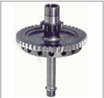
Figure 9—As-received used/scrap carburized AISI 9310 gasifier train gearshaft.
