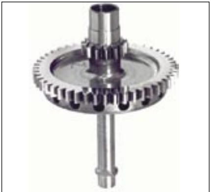
Figure 10—Superfinished used/scrap carburized AISI 9310 gasifier train gearshaft.
