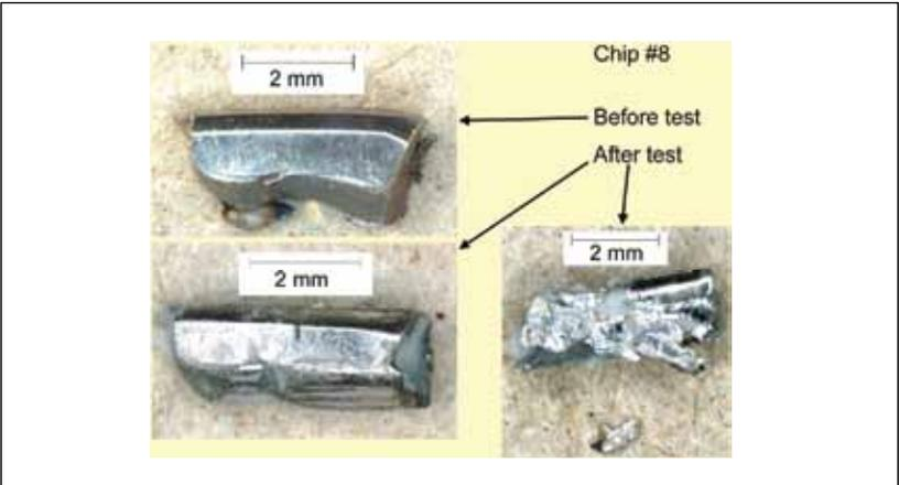
**Figure 16—Chip #8, mass of chip 0.045 grams.**
