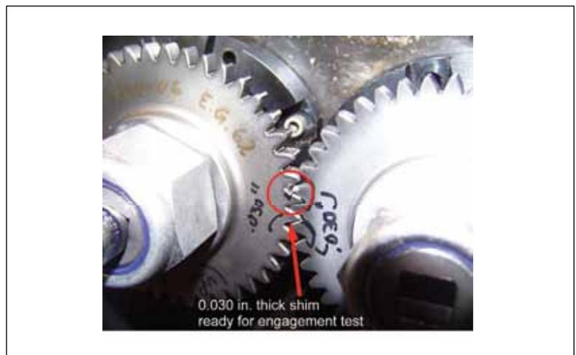
Figure 3—Example of shim and placement used for engagement testing.
