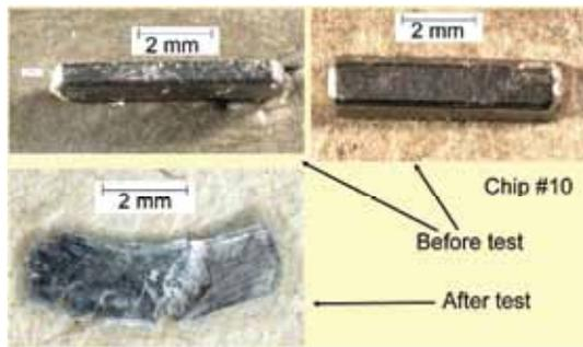
Figure 18—Chip #10, mass of chip 0.032 grams.
