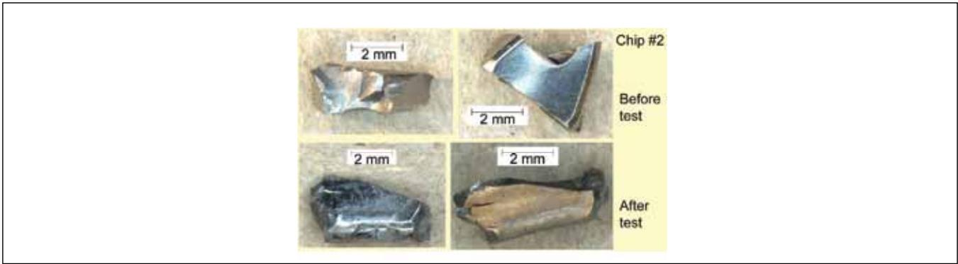
Figure 10—Chip #2, mass of chip 0.100 grams.
