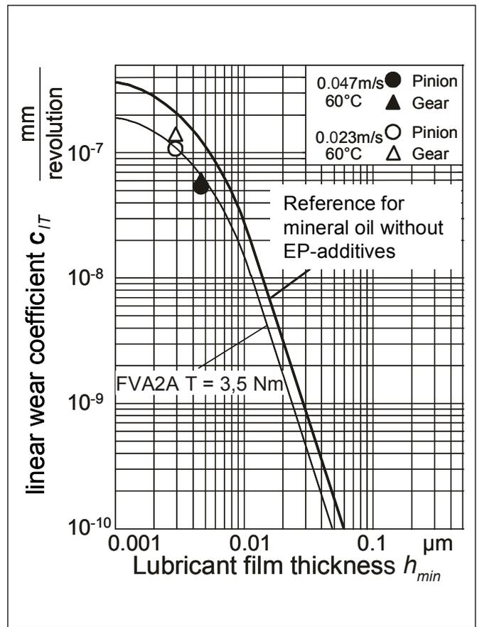
Figure 12—Wear coefficients obtained on FL045 for  $T_1 = 2.85$  Nm.
