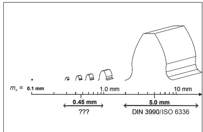
Figure 2—Research area of the present work in comparison to DIN 3990/ISO 6336.
