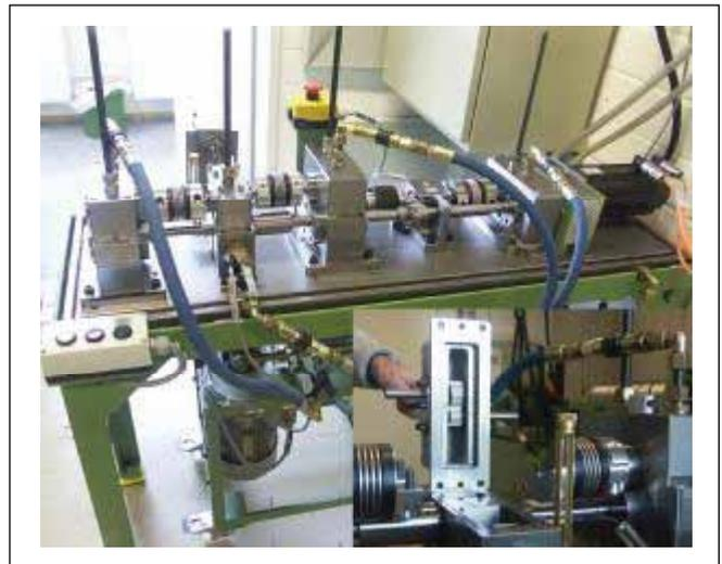
Figure 7—FZG small-size gear test rig.
