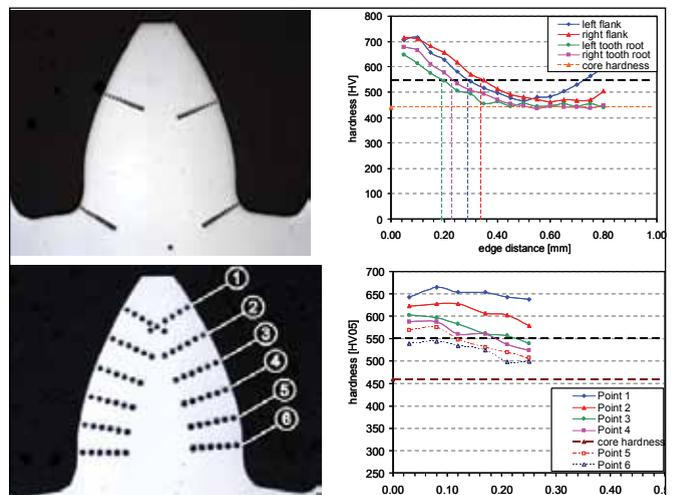
Figure 8—Measurement of the case depth of flank variant test gear (FL06;  $z = 19$ , above) and reference gear (FL045;  $z = 19$ , below) along tooth profile. Case depth graphic of FL045 is an example of one right flank.
