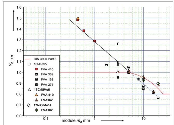
Figure 13—Experiment-derived size factors  $Y_{X', Test}$  against  $Y_{X, DIN/ISO}$  (tooth root bending) for case-hardened steel.
