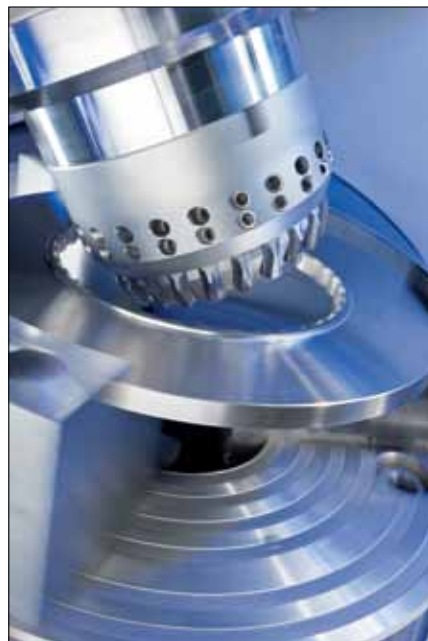
Skiving can be executed on the Oerlikon C29 and C50 bevel gear milling machines. These machines ensure a highly-precise coupling of all movements which are necessary for skiving.
