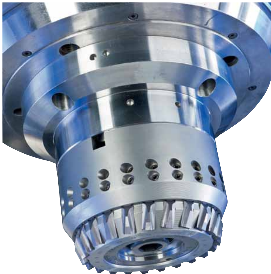
The new stick blade tool system uses carbide technology which has long been used for bevel gears (All photos courtesy of Klingelnberg).
