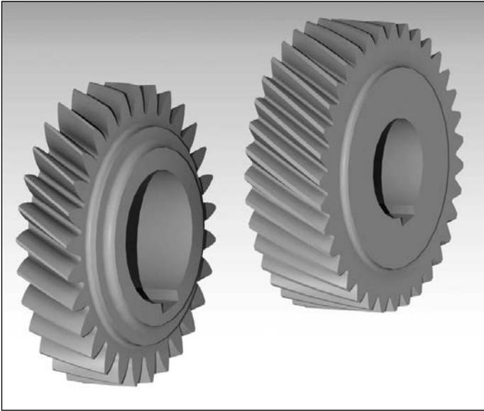
**Figure 3** Conventional and low-loss external gear ( $m_n=2$ ;  $z=35$ ).
