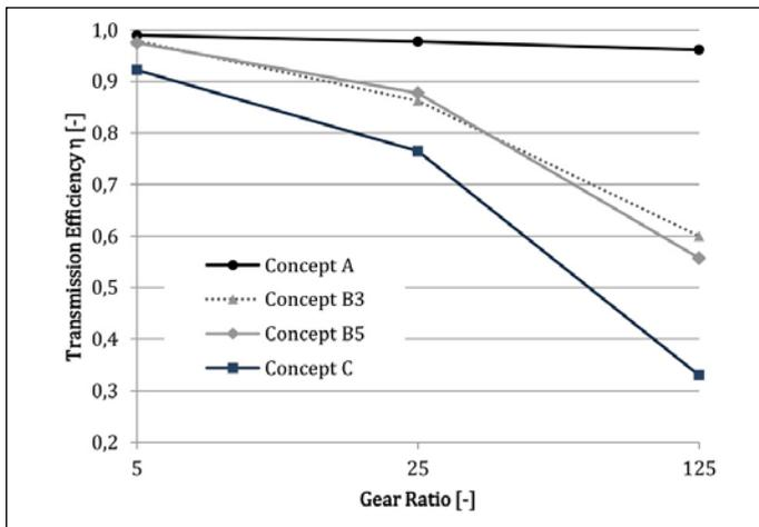
**Figure 7 Efficiency of conventional and low-loss external gear.**
