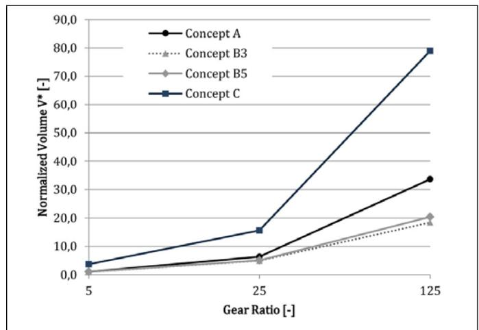
Figure 9 Volume of conventional and low-loss external gear.
