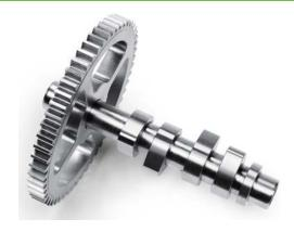
advantages of this process from EMAG also apply to the machining of other components. When machining gear shafts, ground gears can be joined tightly on the shaft, without needing to account for the grinding wheel overrun at the design stage. It also minimizes the length of the shaft and makes the whole unit more compact.
