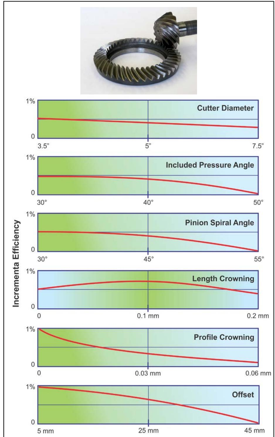
Figure 13 Efficiency influence on test hypoid gearset.
