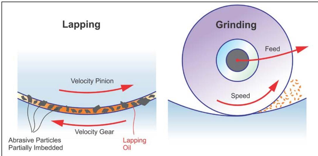
Figure 6 Material removal mechanism: (left) lapping; (right) grinding.
