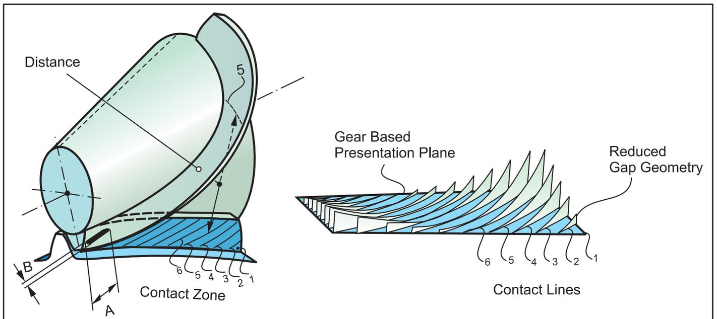
Figure 3 Contact gap and contact geometry aspects (Ref. 2).
