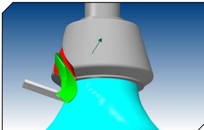
Figure 4 Component clamped in device, deburring tool trajectory in green.
