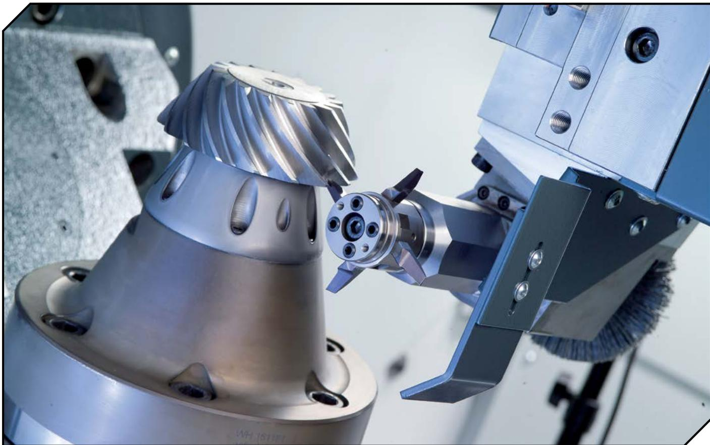
**Deburring or chamfering of gear teeth is gaining attention in practical settings.** And with a view to make the production sequence as efficient as possible, it is becoming increasingly important to be able to implement the deburring tasks directly on the cutting machine after spiral cutting. Read on to find out how complex this seemingly simple task can turn out to be, and how a new deburring concept provides for enhanced efficiency.
