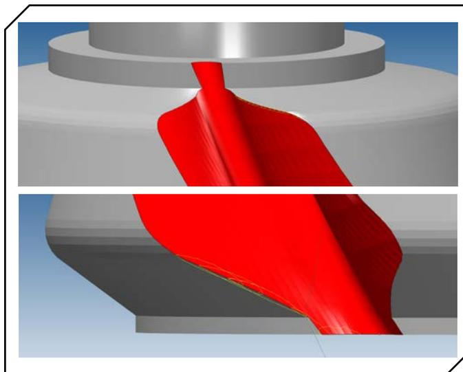
Figure 3 Edges to be deburred, resulting from the cutting area between the component envelope and the component gap.
