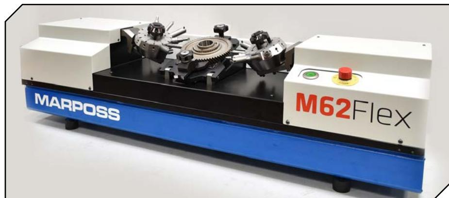
the measuring group is able to approach a gear surface in velocity mode, with a controlled low force, while the position error is monitored, resulting in better control of the process and avoiding
