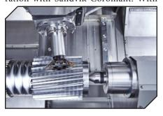
these manufacturing methods, virtually all machining challenges for gear manufacturing can be covered. Moreover, the ability to measure the gears in the machine improves the efficiency and reduces risk of error.
