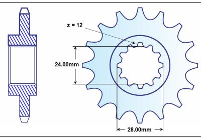
Figure 7 Example sprocket with internal spline.
