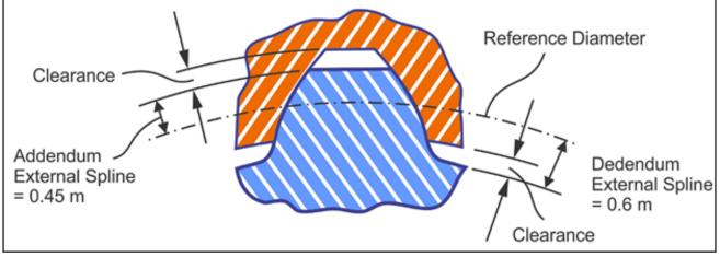
Figure 4 Flank centered connection.
