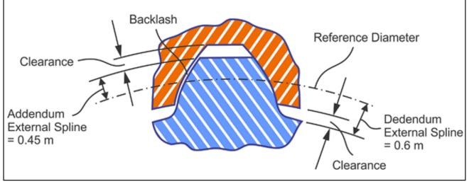
Figure 3 Not centering connection.
