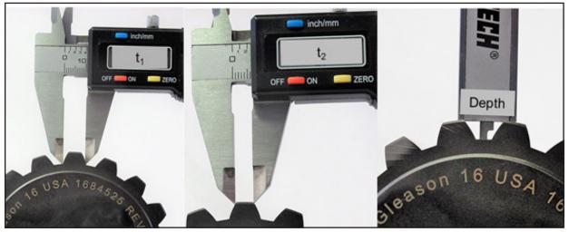
Figure 8 Measurement of topland root and depth.
