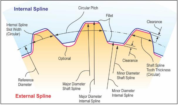
Figure 1 Design parameters for splines.
