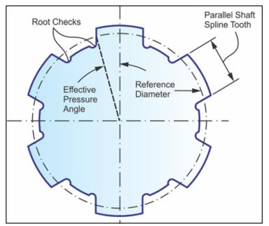
Figure 6 Parallel straight sided spline.
