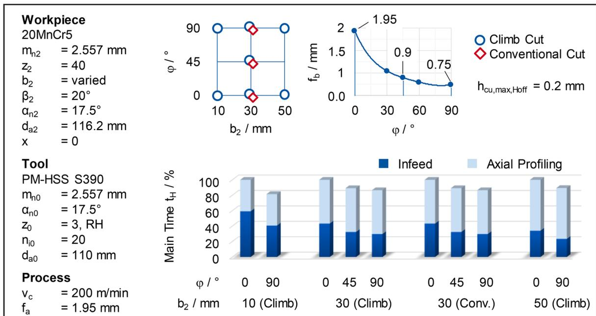
Figure 5 Design of experiments and resulting main times.
