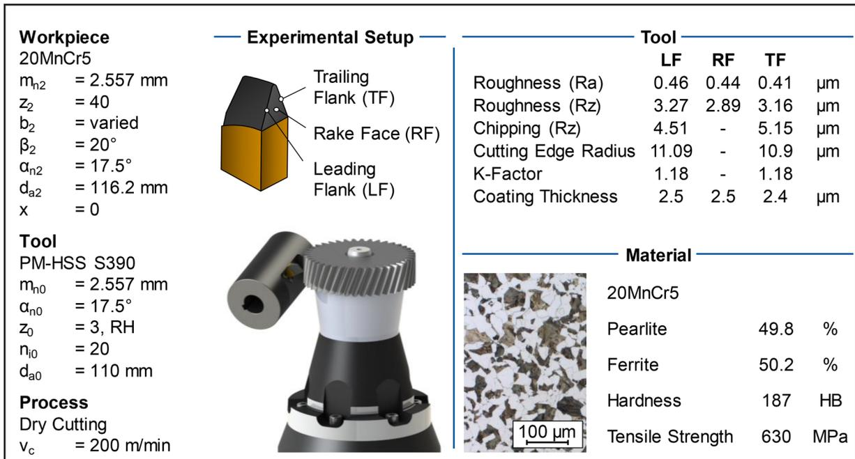
Figure 4 Experimental setup, tool and workpiece characterization.
