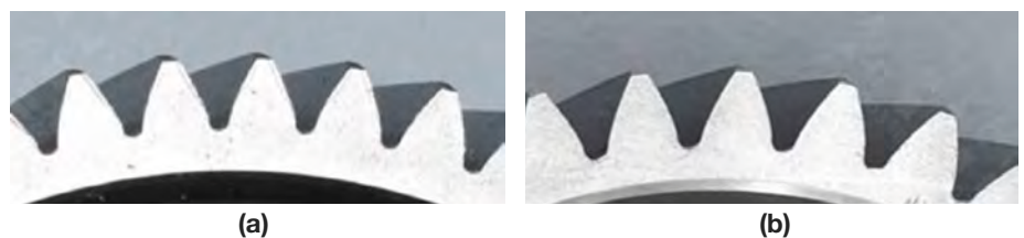
Figure 7—Experimental gears; (a)—with symmetric teeth, (b)—with asymmetric teeth.
