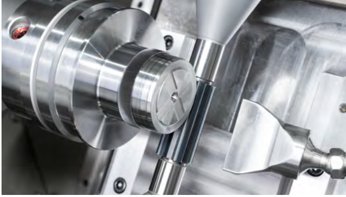
Hobbing of external strain wave gears in robotic gearboxes on 80PS with carbide hob.
