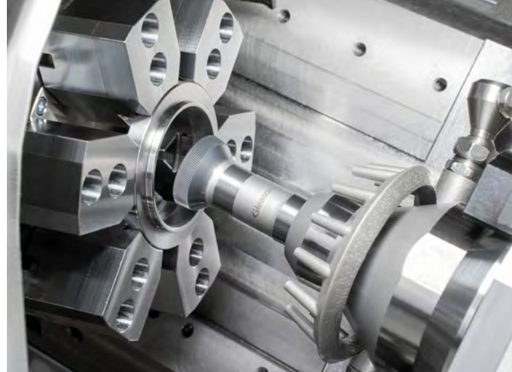
Power skiving of robotic strain wave internal ring gears for robotic gearboxes with carbide cutter.
