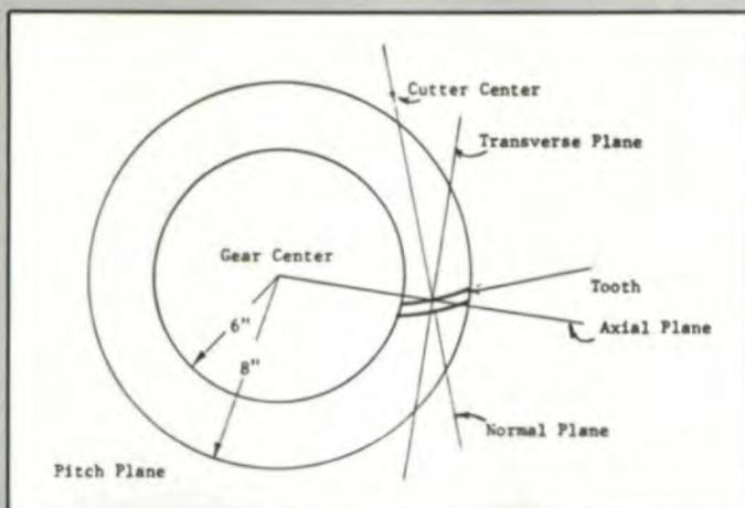
Fig. 1—Spiral Bevel Crown Gear and Identifying Planes
