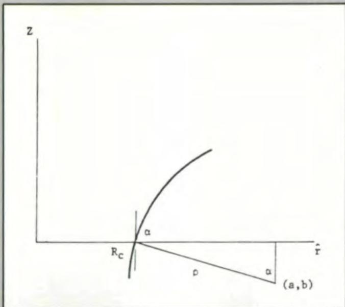
Fig. 7—Circular Tooth Profile in the Normal Plane
