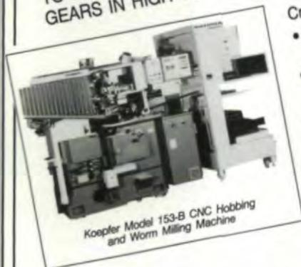
Koepfer Model 153-B CNC Hobbing and Worm Milling Machine
