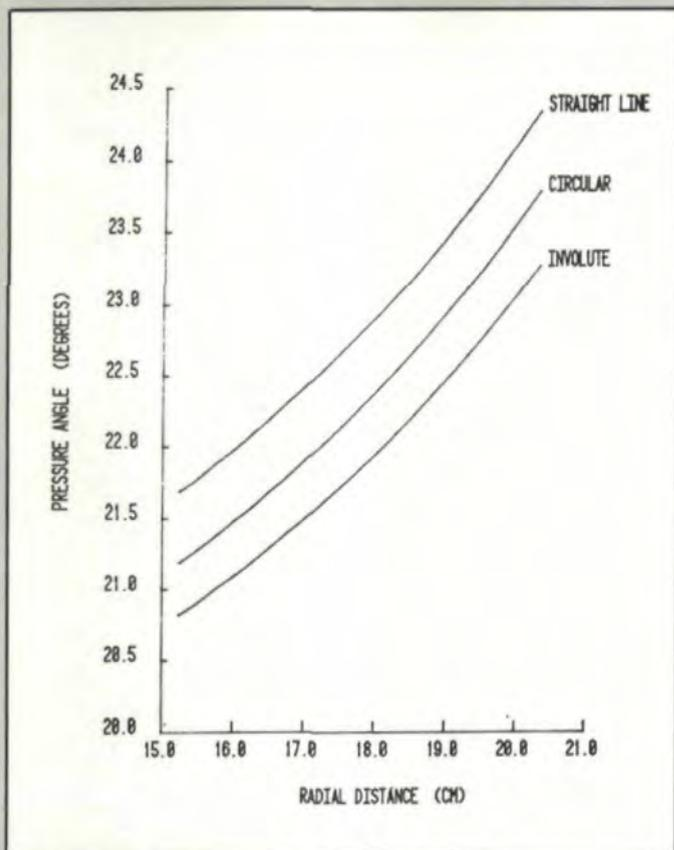
Fig. 9—Pressure Angle Variation for Three Cutter Profiles
