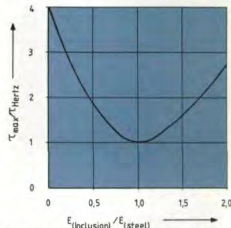
Fig. 2 - The increase in tension in the surroundings of non-metallic inclusions in the process of over-running bearing steel 100 Cr 6. Reference 3: Findings from optical tension model tests in simulating the stress distribution on a contact line of a ball bearing inner ring 6309 for  $F_r = 19200 \text{ N}$  radial load.
