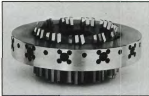
Fig. 10 - Single-part blade head for series manufacture.
