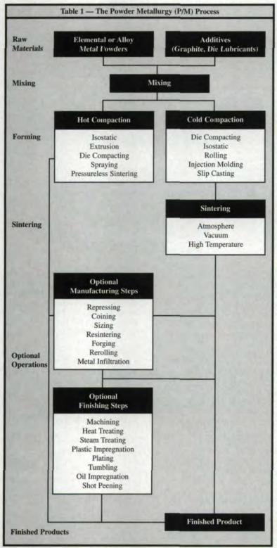
owder metallurgy (P/M) is a precision metal forming technology for the manufacture of parts to net or near-net shape, and it is particularly well-suited to the production of gears. Spur, bevel and helical gears all may be made by powder metallurgy processing.
