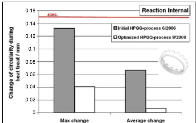
**Figure 15—Maximum and average change of circularity during heat treatment in a load of reaction internal gears; comparison of initial production process from 2006 and the optimized production process used since 2008; specimen maximum after heat treat—150 μm.**
