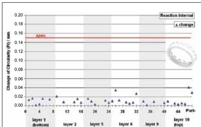
**Figure 13—Change of circularity of reaction internal gears during heat treatment (LPC and HPGQ with dynamic quenching); spec. maximum after heat treat: 150 μm.**
