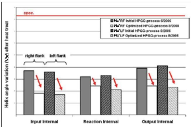
**Figure 16—Helix angle variation after heat treatment averaged per load for input reaction and output internal gears; comparison of initial production process from 2006 and the optimized production process since 2008.**
