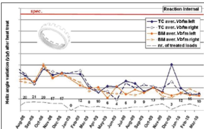
**Figure 17—Reaction internal gears: helix angle variation after heat treat averaged per month of production: (TC = sample from top corner of the load; BM = sample from bottom middle of the load; the number of inspected loads is indicated per each month; the total number of inspected loads from 2008 until 2010 was 229 loads; no production in 2009).**
