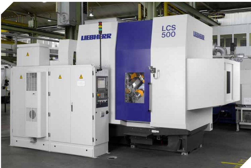
On the LCS 500 gear grinding machine, Liebherr displayed a type of error-proofing called Collision Control which many attendees found valuable (courtesy of Liebherr).
