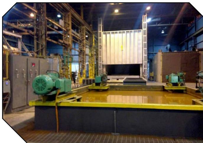
All equipment from both companies has been consolidated at the 65,000 square foot Complete facility in Milwaukee, where the highlight is a gas-fired car bottom furnace with a 53' x 22' x 14' workspace, powered by 40,000,000 BTUs with a 1,000,000-pound load capacity and operating temperatures to 2,150°F max.
