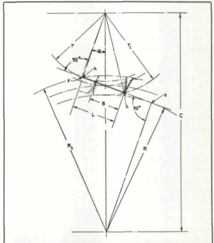
Fig. 9—Diagram illustrating mathematical method for determining actual length of tooth contact.
