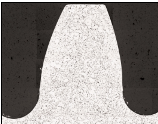
Figure 8—Photomicrograph of rolled densified helical gear tooth taken through crowned section.
