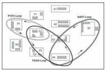
Figure 1—The POLCA system uses production cards circulating between overlapping pairs of workcenters to make most efficent use of production equipment in companies manufacturing custom-engineered and high-variety products.
