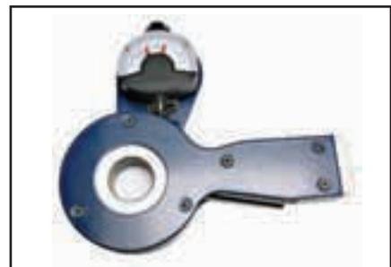
Frenco has expanded its product line by starting to produce a circumferential backlash measuring instrument.
