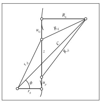
Figure 1—Calculation of contact ratio.
