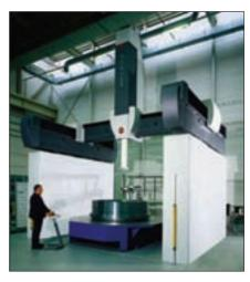
Hexagon Metrology announced the Leitz PMM-G gantry CMM series at Gear Expo 2009, featuring improved specifications and extra size availability, so it's appropriate for highly precise inspection of extremely large components, like gears used for wind power, gear segments, gear racks and geared shafts of up to 5,000 mm in diameter.
