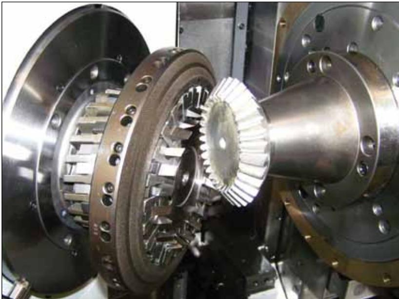
Figure 6—Zerol bevel gear cutting.
