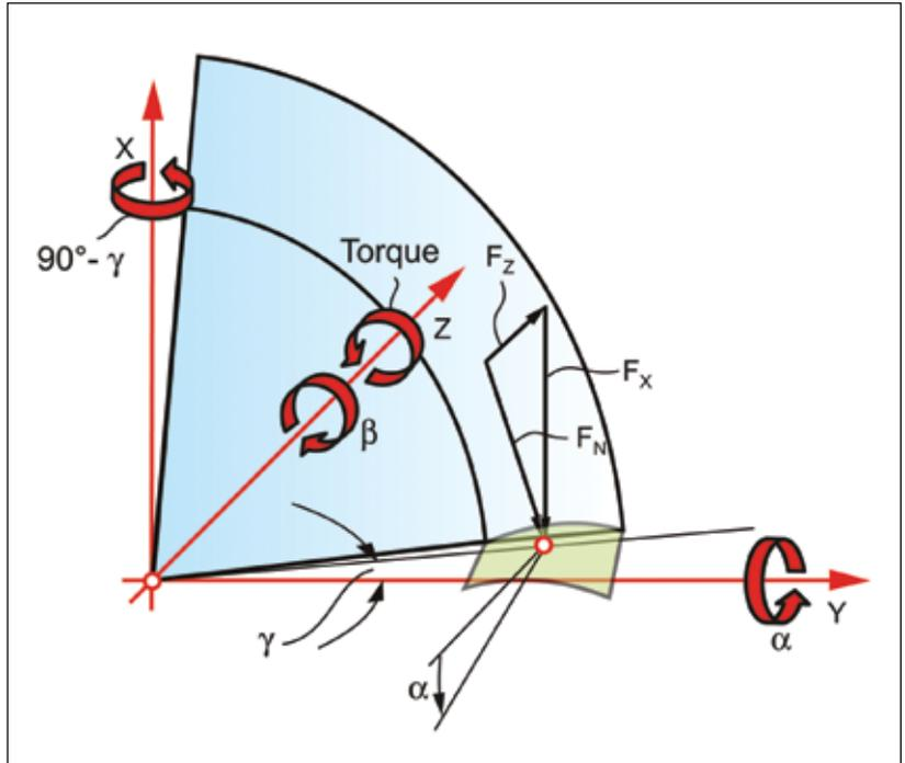
Figure 8—Force diagram for calculation of bearing loads.
