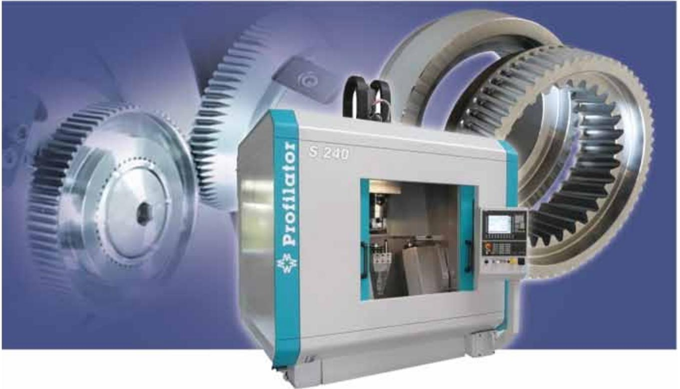
This revolutionary process called Scudding®, developed by Wera Profilator GmbH, involves a machine using synchronized spindles and a HSS cutter that feeds directly *through* the work piece to generate a high-quality gear – internal or external, spur or helical.
