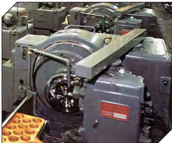
Figure 1 Gleason No. 116 bevel and hypoid gear generator.
