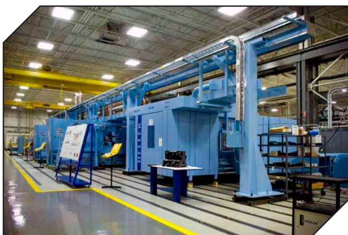
iron, a very hard material cast into large diesel engine blocks. Machining CGI requires a very stable, heavy-duty machine tool, and Heller CGI machining centers have been placed in nearly all heavy-duty diesel engine and others.
